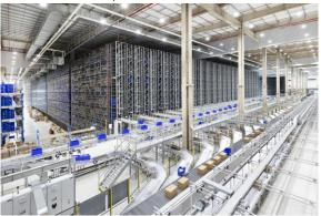
for material flow from goods receiving to multi-shuttle storage systems, order picking and automatic palletising.
